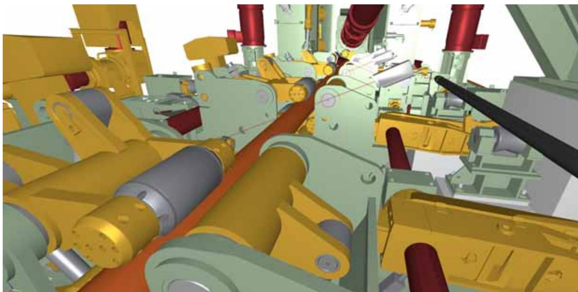
*3D model for real-time simulation of a seamless tube plant according to the Mannesmann principle including the forming process for a product*
